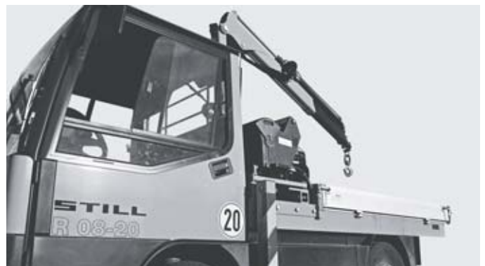
Optional built-in crane for lifting heavy loads
