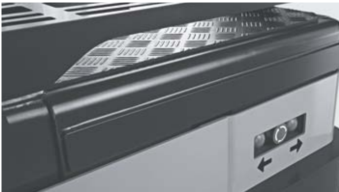
Reversing device for driving safely and precisely up to the trailer
