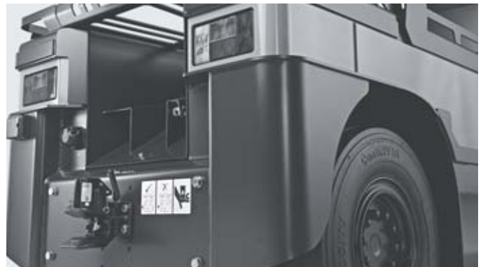
R 07 electric tractor: trailer coupling for use as a towing vehicle
