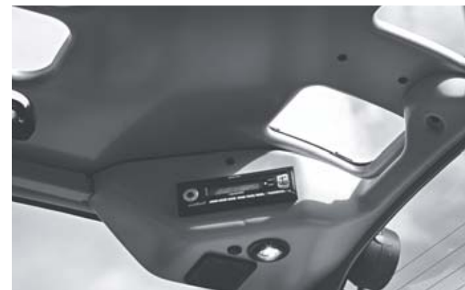
Viewing window also to the top rear in order to prevent roller shutter damage
