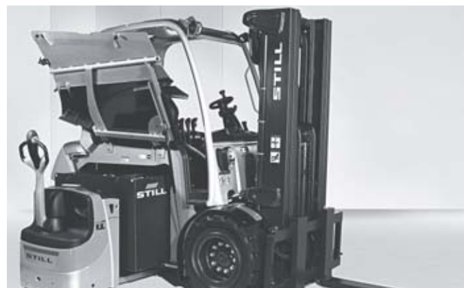
Simple lateral battery changing with pallet truck and battery bed
